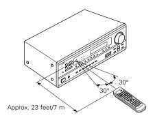
Point the remote control unit at the remote control sensor as shown on the diagram at the left.
